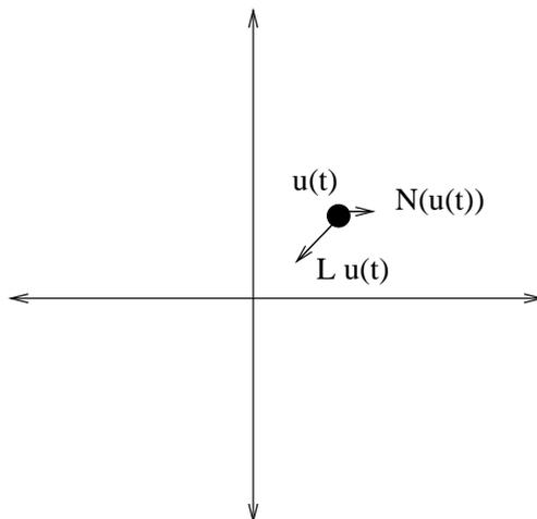
FIGURE 14. Proposition 1.41 from the vector field perspective of Figure 1. If  $u$  is sufficiently small, then the dissipative effect of the linear term  $Lu$  will dominate the effect of the nonlinearity  $N(u)$ , regardless of the orientation of  $N(u)$ , causing  $u$  to decay exponentially towards the origin.
