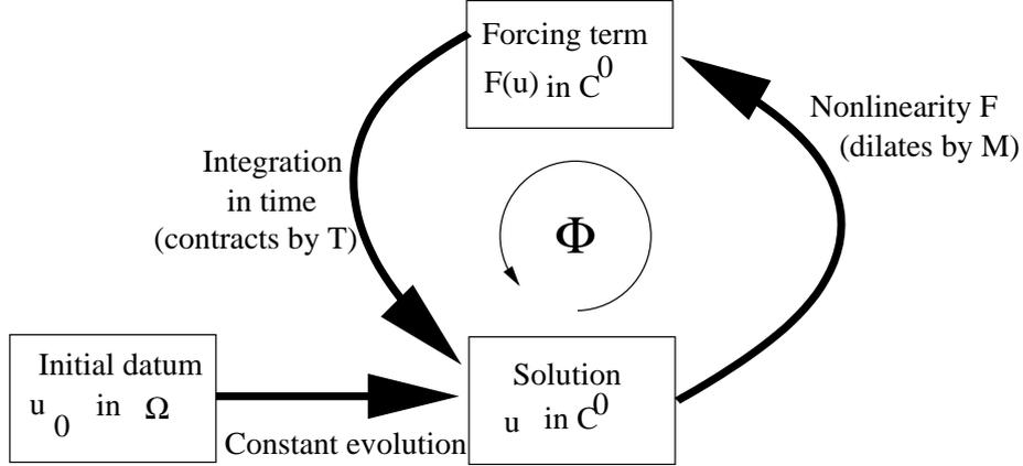
FIGURE 3. The Picard iteration scheme. The map  $\Phi$  is basically the loop from the solution  $u$  to itself. To obtain the fixed point, start with the initial datum  $u_0$  as the first approximant to  $u$ , and apply  $\Phi$  repeatedly to obtain further approximations to  $u$ . As long as the net contraction factor  $T \times M$  is less than 1, the iteration scheme will converge to an actual solution.
