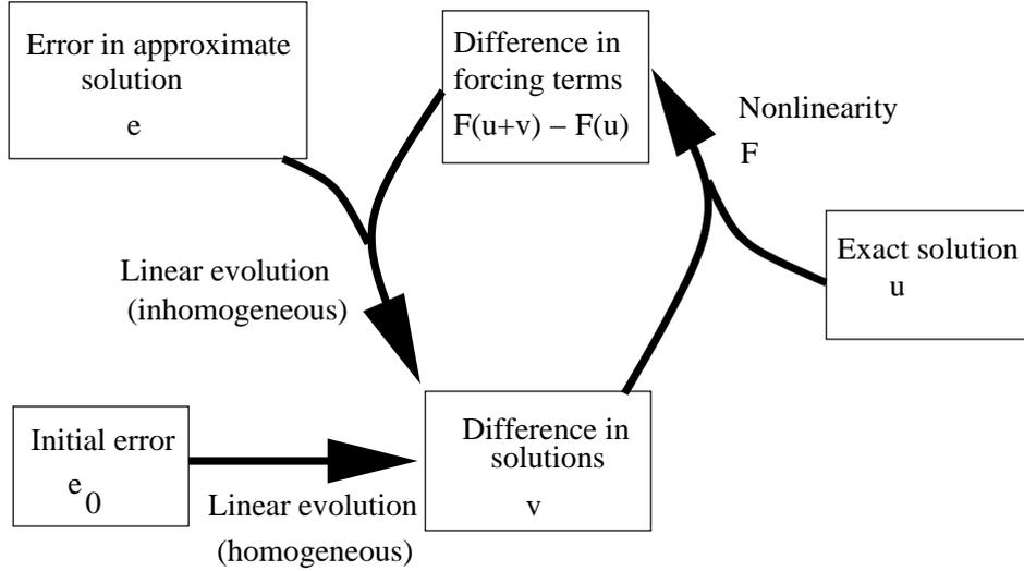
FIGURE 10. The difference scheme for an approximate perturbation  $\tilde{u} = u + v$  to an exact solution  $u$ . This scheme can also be reversed to convert an approximate solution  $\tilde{u}$  to an exact solution  $u = \tilde{u} - v$  (by replacing  $F(u + v) - F(u)$  with  $F(\tilde{u}) - F(\tilde{u} - v)$ ).
