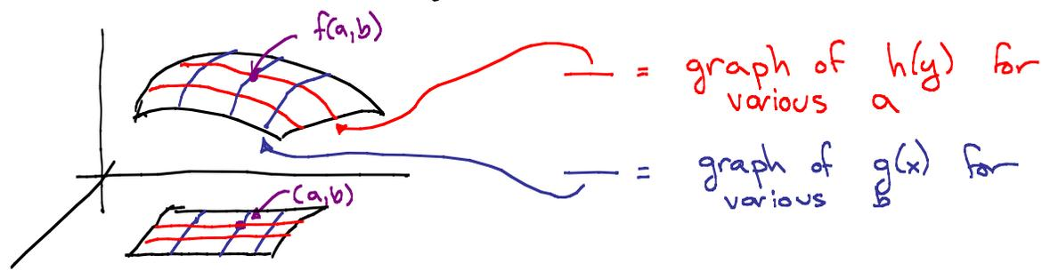
So  $f_y(a,b)$  is the slope of the tangent line to the red curve through  $(a,b)$ , while  $f_x(a,b)$  is the slope of the tangent line to the blue curve through  $(a,b)$ .
