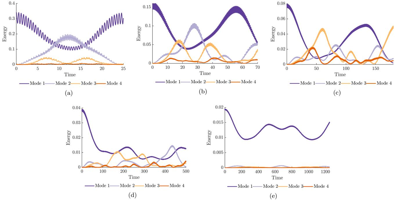
FIG. 9. Simulations of 1D FPUT- $\alpha$  arrays with different numbers of oscillators ( $N$ ) at a tolerance of  $\pm 5\%$  with a coupling coefficient of  $\alpha = 0.25$ . (a)  $N = 8$ , (b)  $N = 16$ , (c)  $N = 32$ , (d)  $N = 64$ , and (e)  $N = 128$ . [Panel (d) appeared previously in Fig. 8(b).]
