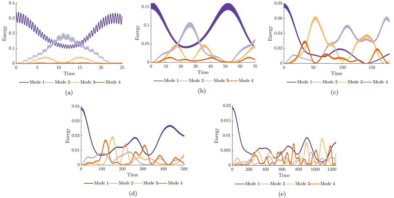
FIG. 6. Simulations of 1D FPUT- $\alpha$  arrays with different numbers of oscillators ( $N$ ) at a tolerance of  $\pm 5\%$  with a coupling coefficient of  $\alpha = 0.25$ . (a)  $N = 8$ , (b)  $N = 16$ , (c)  $N = 32$ , (d)  $N = 64$ , and (e)  $N = 128$ . [Panel (d) appeared previously in Fig. 5(b).] This figure illustrates that, for a given tolerance, arrays with fewer oscillators are more likely to exhibit recurrence (which does not occur if there are too many oscillators).
