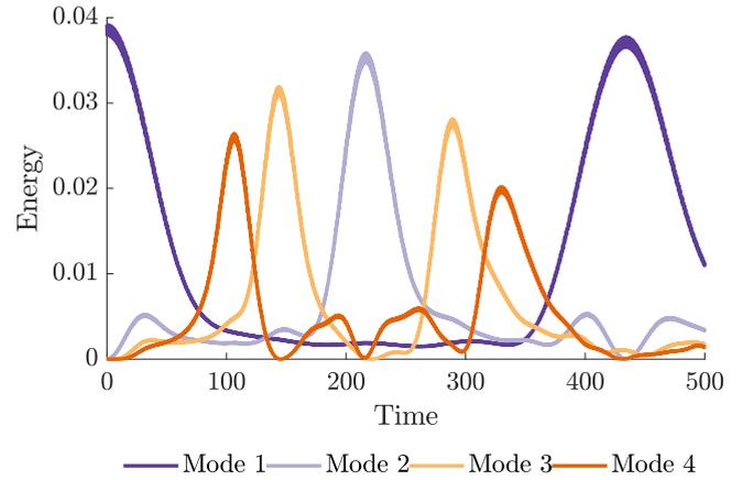
FIG. 4. Simulation of a 1D FPUT- $\alpha$  array with symmetric tolerances, 64 oscillators, and a coupling coefficient of  $\alpha = 0.25$  at a tolerance of  $\pm 0.1\%$ . Comparing this to Fig. 2, we see a slight variation from the response of an ideal system.
