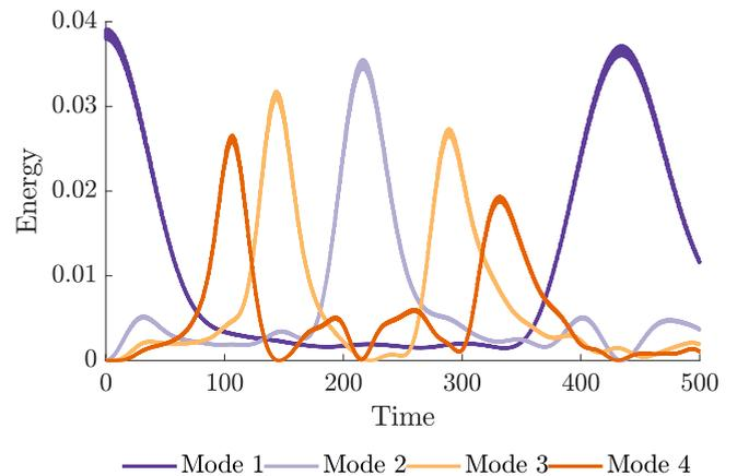
FIG. 7. Simulation of a 1D FPUT- $\alpha$  array with asymmetric tolerances, 64 oscillators, and a coupling coefficient of  $\alpha = 0.25$  at a tolerance of  $\pm 0.1\%$ . Comparing this simulation to that in Fig. 4, we observe that this asymmetric system has a comparable deviation from ideal recurrence (i.e., when there is no tolerance) to the symmetric system.
