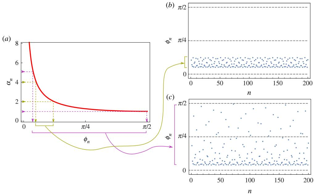
**Figure 2.** (a) Interaction coefficient  $\alpha_n$  for model II as a function of the contact angle  $\phi_n$  between adjacent cylinders. (b,c) The contact-angle distributions for two cases: (i)  $\bar{\alpha}_1 = 3$  and  $\bar{\alpha}_2 = 1$ ; and (ii)  $\bar{\alpha}_1 = 3$  and  $\bar{\alpha}_2 = 3$ . We use arrows to represent the mapping process that we describe in the text. (Online version in colour.)
