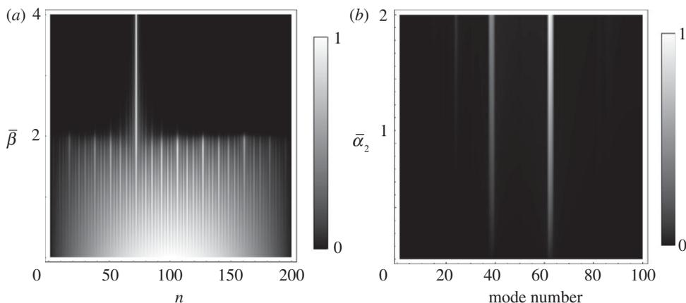
**Figure 4.** (a) Localization transition, as evidenced by the absolute value of the amplitude  $u_n$  for each  $n$ , as a function of  $\bar{\beta}$  for the fundamental mode in model Ia with  $N = 200$  particles. (b) Inverse participation ratio as a function of  $\bar{\alpha}_2 \in [0, 2]$  (and with  $\bar{\alpha}_1 = 3$ ) for model II with  $N = 100$  cylindrical particles.
