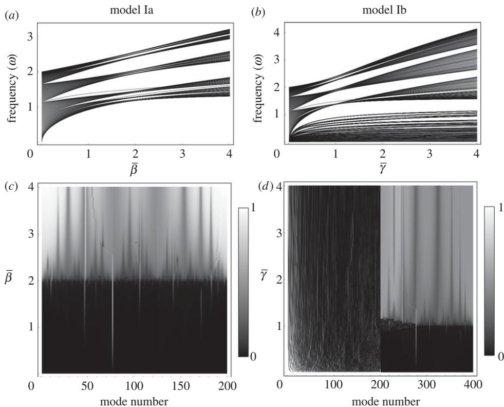
**Figure 3.** (a,b) Linear spectrum of models Ia and Ib as a function of the quasiperiodicity parameter and (c,d) inverse participation ratio (IPR) as a function of mode number and the quasiperiodicity parameter for the two models. We show our results for model Ia in panels (a,c) and for model Ib in panels (b,d).
