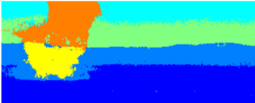
Fig. 4 Segmentation of a hyperspectral video using graph MCF. The gas plume is clearly represented in the yellow and orange pixels. The two blue communities on the bottom are the ground, and the other two communities are the sky. This image is frame 3 of 7. (It is best to view this plot in color.) (Color figure online)
