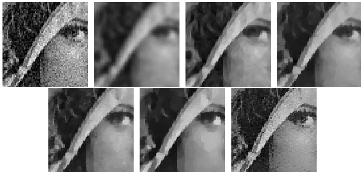
FIG. 3. Denoising experience on a natural image. From left to right and from top to bottom: noisy image (standard deviation 20), Gaussian convolution, anisotropic filter, total variation minimization, Tadmor-Nezzar-Vese iterated total variation, Osher et al. iterated total variation, and the Yaroslavsky neighborhood filter.
