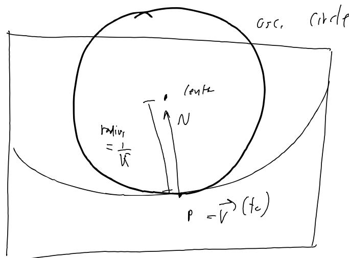
$$(r_{\text{center}}, \vec{r}(t_0) + \frac{1}{k(t_0)} \vec{N} \theta_0)$$
