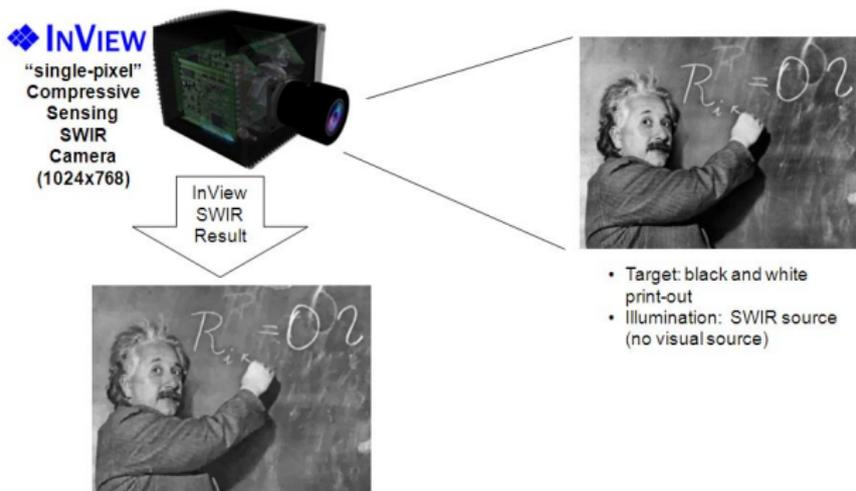
Figure: SWIR Reconstruction using  $m = .5N^2$  measurements
