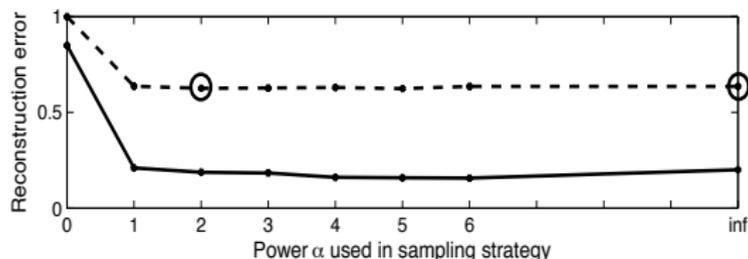
(a) Reconstruction errors by various power-law density sampling at low noise (filled line) and high noise (dashed line)
