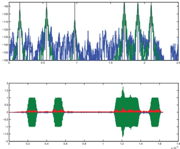
Figure: Recovery in both the time (below) and frequency (above) domains by  $\ell_1$ -analysis. Blue denotes the recovered signal, green the actual signal, and red the difference between the two.
