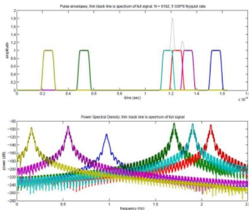
Figure: The signal is a superposition of 6 radar pulses, each of which being about 200 ns long, and with frequency carriers distributed between 50 MHz and 2.5 GHz (top plot). As can be seen, three of these pulses overlap in the time domain
