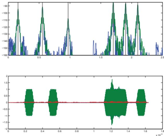
Figure: Recovery in both the time (below) and frequency (above) domains by  $\ell_1$ -analysis after one reweighted iteration. Blue denotes the recovered signal, green the actual signal, and red the difference.
