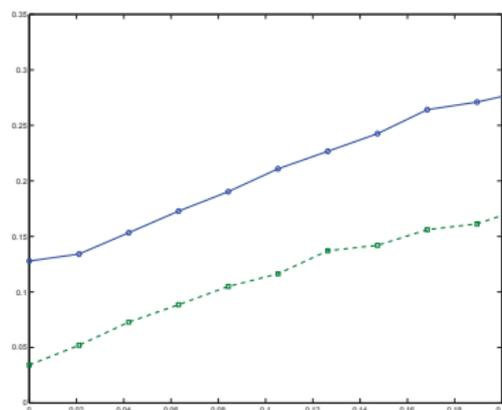
Figure: Relative recovery error of  $\ell_1$ -analysis as a function of the (normalized) noise level, averaged over 5 trials. The solid line denotes standard  $\ell_1$ -analysis, and the dashed line denotes  $\ell_1$ -analysis with 3 reweighted iterations. The x-axis is the relative noise level  $\sqrt{m}\sigma/\|Af\|_2$  while the y-axis is the relative error  $\|\hat{f} - f\|_2/\|f\|_2$ .
