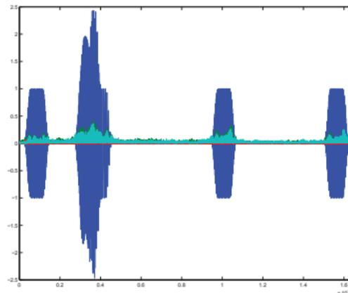
Figure: Relative error  $\|\hat{f} - f\|_2 / \|f\|_2$  of a compressible signal. Blue denotes the actual signal, while green, red, and cyan denote the recovery error from  $\ell_1$ -analysis, reweighted  $\ell_1$ -analysis, and  $\ell_1$ -synthesis, respectively.
