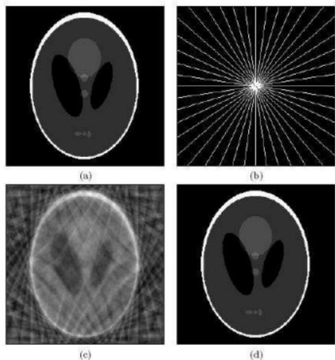
Figure 1: Example of a simple recovery problem. (a) The Logan-Shepp phantom test image. (b) Sampling domain  $\Omega$  in the frequency plane; Fourier coefficients are sampled along 22 approximately radial lines. (c) Minimum energy reconstruction obtained by setting unobserved Fourier coefficients to zero. (d) Reconstruction obtained by minimizing the total variation, as in (1.1). The reconstruction is an exact replica of the image in (a).
