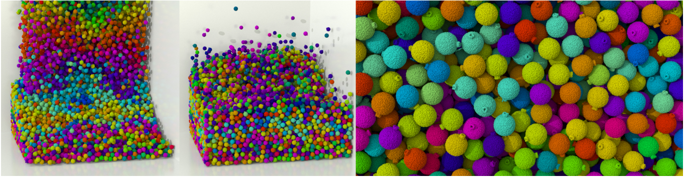
Fig. 2. Bomb falling. We run the bomb falling test on 8 GPUs with 134M particles (6,688 bombs with nonlinear finite-strain hyperelastic constitutive models) and grid resolution 512 \times 2048 \times 512 . On average, each frame is finished within 1 minute, indicating the scalability of our proposed multi-GPU MPM pipeline.
