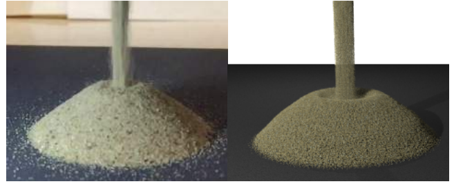
Figure 12: Sand is poured from a spout into a pile in a lab (left) and with our method (right).
