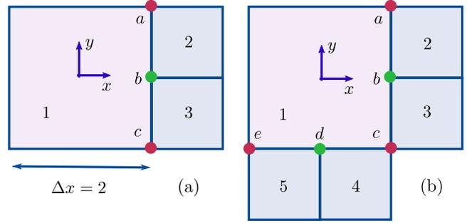
Fig. 5. **Illustration of free T-junction.** A test case for the adaptive grid basis with free T-junctions described in Section 5.1. The interpolation functions remain non-negative in the case of (a). However, in the (b) case where there exist two T-junction nodes,  $N_c$  may turn negative and become problematic.
