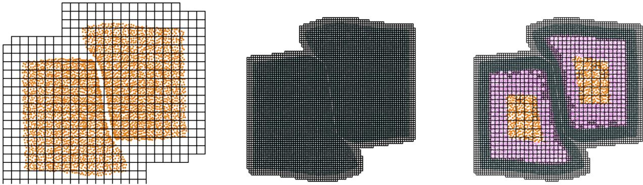
Fig. 4. **Colliding 2D jello squares.** Two hyperelastic jello squares are driven to collide with each other. Left: A uniformly coarse grid leaves large separation gaps. Middle: A 4 $\times$ -refined uniform grid nicely resolves the contact, at the expense of gratuitous computation in the interior. Right: Our adaptive scheme.
