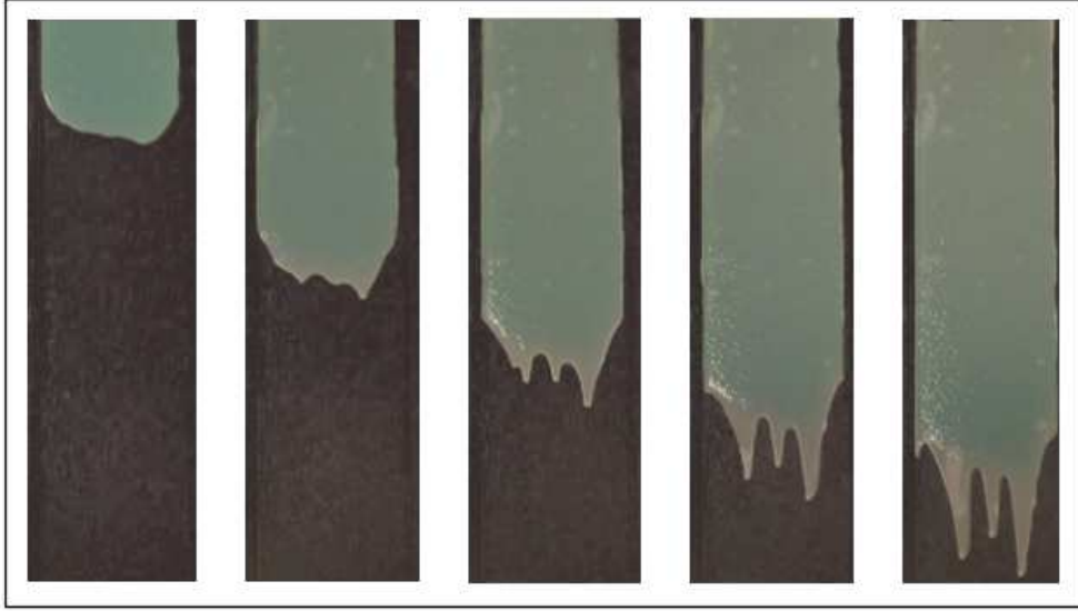
Fig. 9 Pictorial evolution of the ‘settled’ regime showing the particles settling while clear fluid flows over the particles resulting in the formation of fingers. The plane angle of inclination is set to 30^\circ while the particle concentration is chosen as 0.25. The first snapshot is shown 30 seconds after the onset of the experiment while the last one is shown after 3 minutes. The color of the inclined plane has been darkened to clearly show the contrast between the particle-rich region (blue-green) and the clear fluid fingers.
