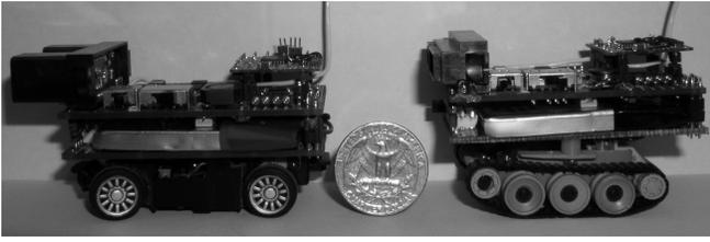
Fig. 2. (left) Car based vehicle. (right) tank based vehicle.
