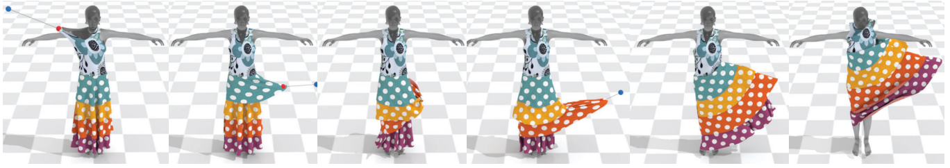
Fig. 14. Tiered skirt. Our method also produces high-quality interpenetration-free cloth animations. The tiered skirt has over 91K simulation DOFs and multiple layers. Our solver robustly resolves all the collisions and self-collisions of the skirt. The simulation FPS is between 12.2 to 29.1.
