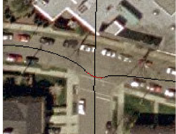
Figure 6.2 The 2 pieces of road separated by the vertical road would not be considered for a possible connection if the Bresenham test were used. When omitted, the linear model detects the gap.
