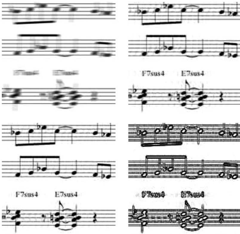
■ Fig. 25-14 The case of a known (nine-pixel horizontal motion) blur kernel. Top-left : corrupted image. Top-right : restoration using the TV method [74, 85]. Bottom-left : restoration using the MS method. Bottom-right : Edge map produced by the MS method
