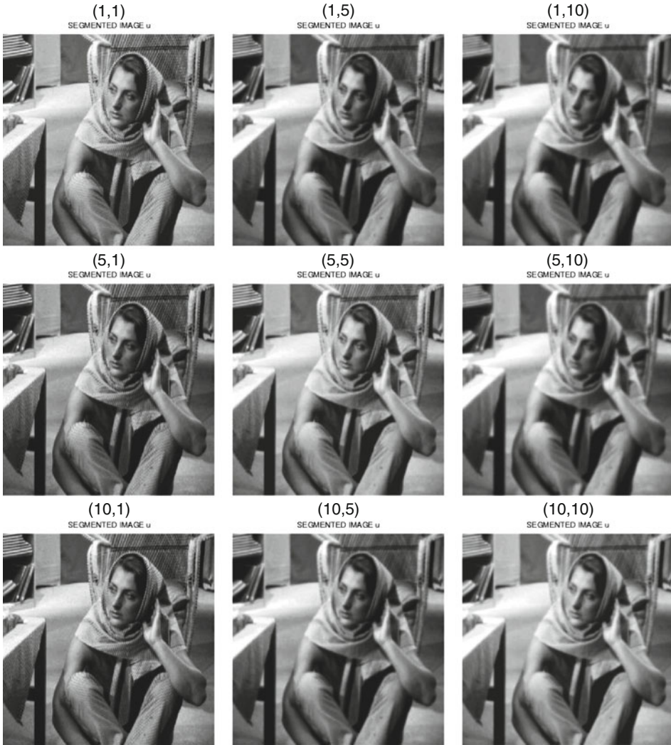
■ Fig. 25-2 Piecewise-smooth images u as minimizers of the Ambrosio–Tortorelli approximations for \epsilon = 0.0001 and various values of (\alpha, \beta)
