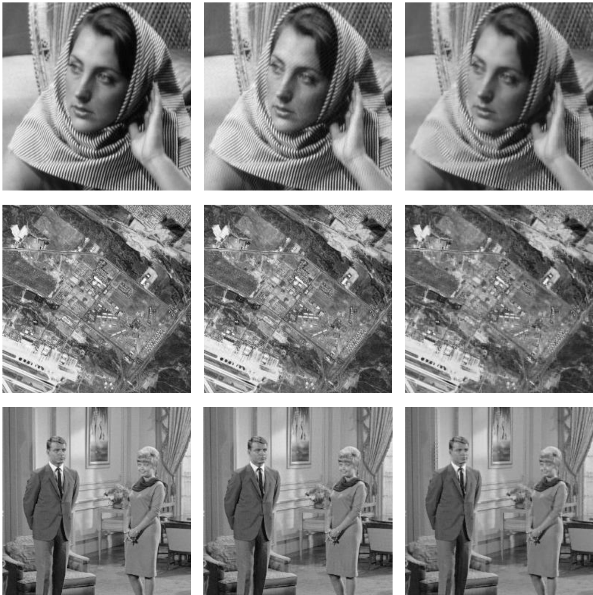
Figure 3. Recovered images: Left - Original. Middle - using TV/Sobolev model. Right - using the Rudin-Osher model 24 .
