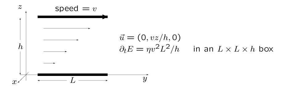
∴  $\eta$  = power required (per area of plate) to maintain unit speed difference across a film of unit width =  $1.0 \times 10^{-4}$  Nm<sup>-2</sup>s for water 20°C
