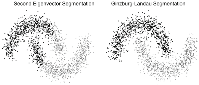
FIG. 4.2. The left-hand figure is the segmentation achieved by thresholding the second eigenvector of the graph Laplacian. The right-hand image is the segmentation obtained from the algorithm presented in this paper. This algorithm segmented the two moon dataset with an error rate of 2.1%.
