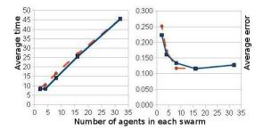
Figure 5: Average detection time (left) and average error (right) as a function of the number of agents in each swarm for case 2 (5 targets and time limit 200.0). The continuous line is for the divide-and-conquer tactic, and the dashed line is the for the results without divide-and-conquer.
