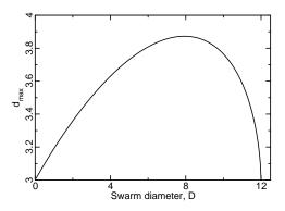
Figure 10: Parameter  $d_{\text{max}}$  versus D for  $r_s = 3.0$ . Note that  $d_{\text{max}}$  increases at first, as the growing size of the swarm allows it to be further away while still easily satisfying (22). However, after the peak at  $D_{\text{opt}} \approx 8$ , condition (22) becomes the limiting factor, requiring greater overlap between the two areas for detection to occur.
