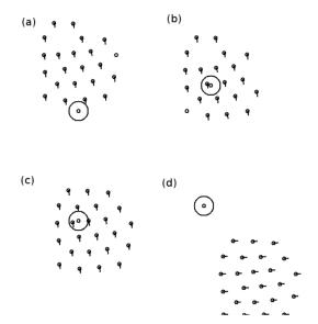
Figure 9: When  $r_s$  is too small compared to D, the swarm does not detect the target. Snapshots (a)-(d) show the swarm flying over the target without locating it. Here N = 24,  $r_s = 1.5$ , required percentage for consensus is p = 25%, and D stabilizes at  $\approx 13.5$ .
