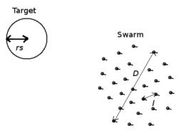
Figure 6: Scales influencing target-locating time: the swarm diameter D, inter-agent length l, and sensing radius  $r_s$ .
