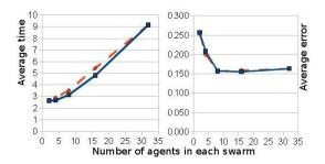
Figure 4: Average detection time (left) and average error (right) as a function of the number of agents in each swarm for case 1 (20 targets and time limit 50.0). The continuous line is for the divide-and-conquer tactic and the dashed line is for the results without divide-and-conquer.
