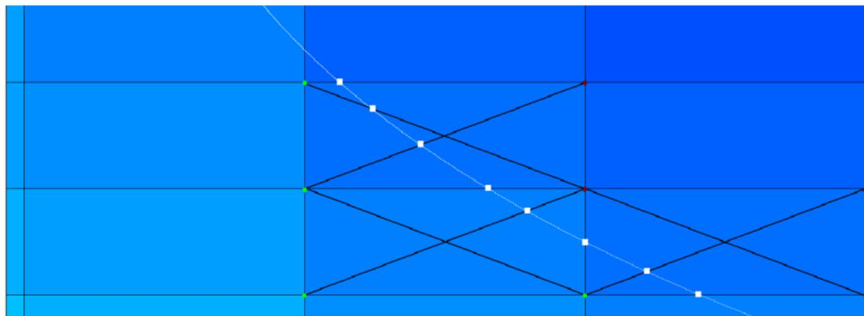
**GREEN dots** mark exterior grid points, **RED dots** mark interior grid points. Unless a grid cell has unanimous sign on all grid points, linearly interpolate the zero-crossing on each of the 6 edges.
