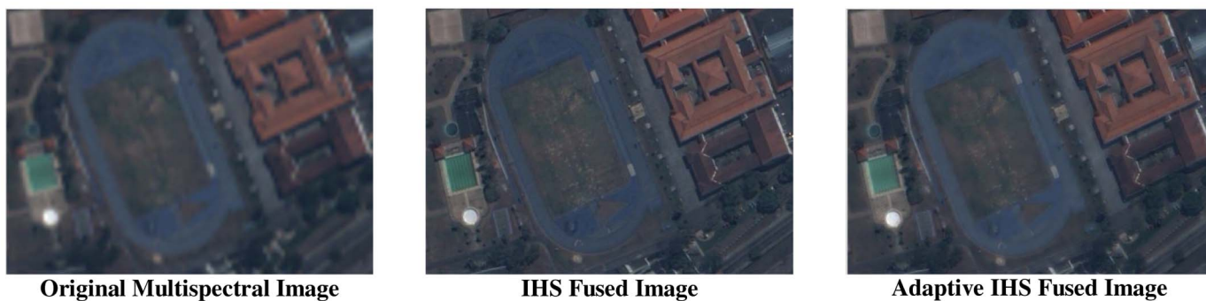
Fig. 2. Pan-sharpening an urban QuickBird scene. Copyright DigitalGlobe, NextView license, 2003.
