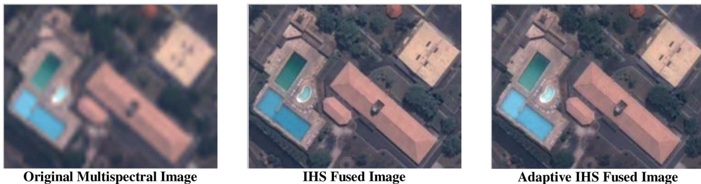
Fig. 1. Pan-sharpening a suburban QuickBird scene. Copyright DigitalGlobe, NextView license, 2003.
