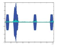
Figure: Relative error  $\|\hat{f} - f\|_2 / \|f\|_2$  of a compressible signal. Blue denotes the actual signal, while green, red, and cyan denote the recovery error from  $\ell_1$ -analysis, reweighted  $\ell_1$ -analysis, and  $\ell_1$ -synthesis, respectively.
