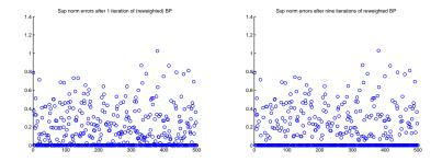
Figure:  $\ell_\infty\text{-norm}$  error for reweighted L1 in the noise-free case
