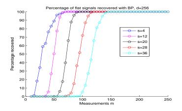
Figure: The percentage of sparse flat signals exactly recovered by Basis Pursuit as a function of the number of measurements *m* in dimension d = 256 for various levels of sparsity *s*.
