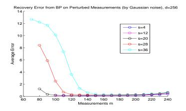
Figure: The recovery error of L1-Minimization under perturbed measurements ( $||e||_2 = 0.5$ ) as a function of the number of measurements *m* in dimension *d* = 256 for various levels of sparsity *s*.  $\equiv -9$  and = -9
