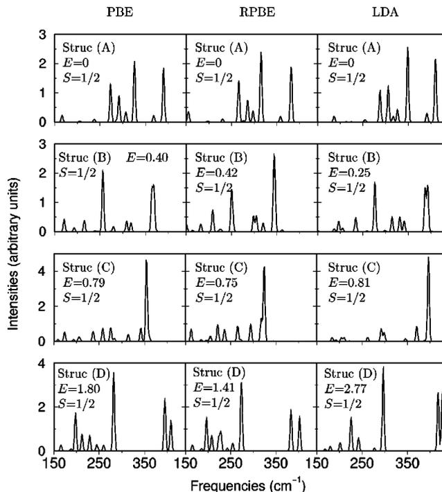
FIG. 2. Comparison of IR spectra for the four most relevant structures for  $V_5^+$  obtained with the GGA within the PBE (left) and the RPBE (middle) parametrization, as well as with the LDA (right). The relative energies are given in eV. Note that no scaling factor has been applied.
