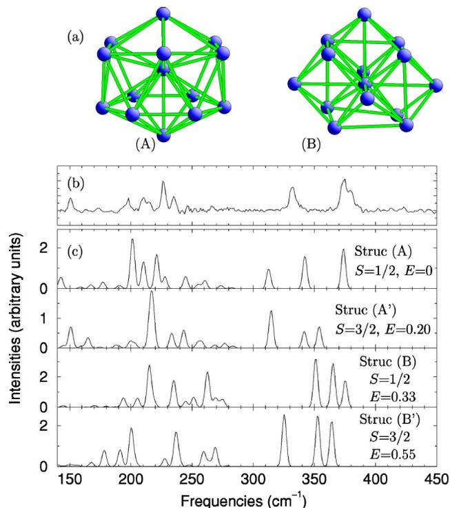
FIG. 17. Results for  $V_{14}^+$ . (a) Schematic representation of the two most stable structures (A)–(B); (b) the spectrum measured experimentally; (c) the spectrum calculated for the structures (A)–(B). The energy differences shown are in eV.
