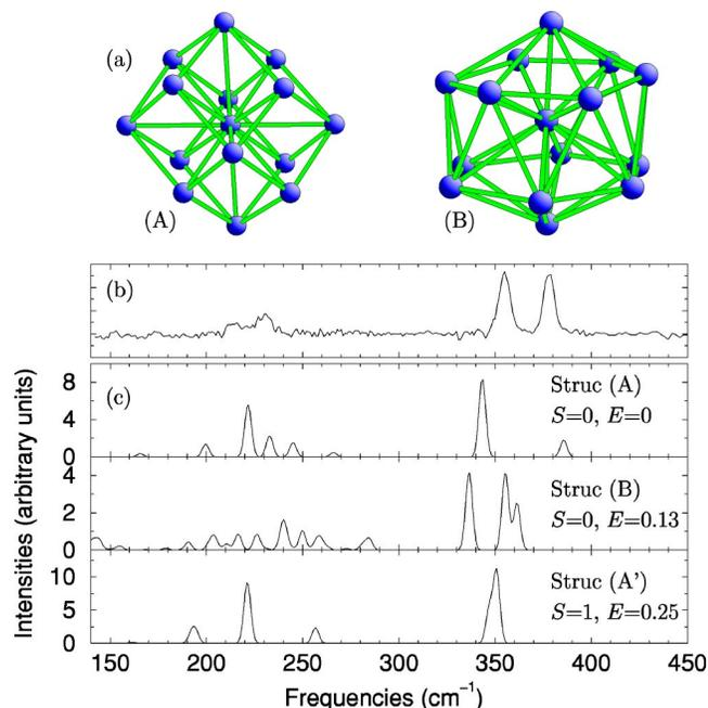
FIG. 18. Results for  $V_{15}^+$ . (a) Schematic representation of the two most stable structures (A)–(B); (b) the spectrum measured experimentally; (c) the spectrum calculated for the structures (A), (B), and (A'). The energy differences shown are in eV.
