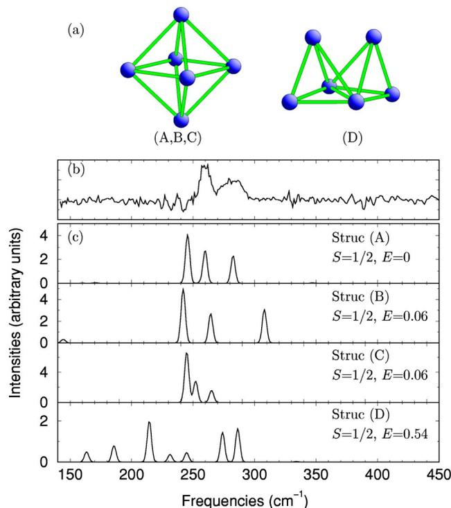
FIG. 8. Results for  $V_6^+$ . (a) Schematic representation of the four most stable structures ( $A$ )–( $D$ ). Since structures ( $A$ )–( $C$ ) are very similar (and only differ slightly in bond lengths), only one picture is shown; (b) the spectrum measured experimentally for  $V_6Ar_2^+$ ; (c) the spectrum calculated for the structures ( $A$ )–( $D$ ). The energy differences shown are in eV.
