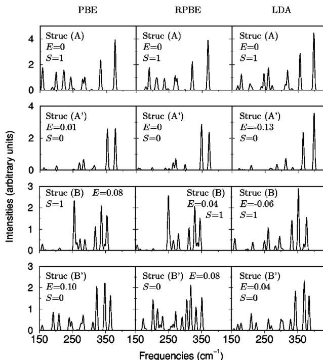
FIG. 3. Comparison of IR spectra for the four most relevant structures for  $V_5^+$  obtained with the GGA within the PBE (left) and the RPBE (middle) parametrization, as well as with the LDA (right). The relative energies are given in eV. Note that no scaling factor has been applied.
