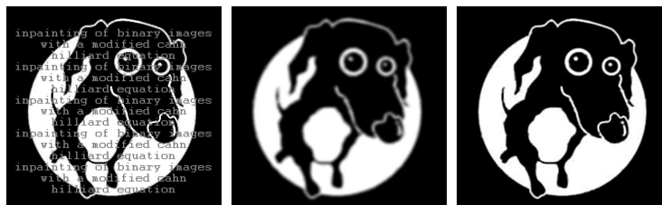
FIGURE 4. Text removal from a binary image: the solution of Cahn-Hilliard inpainting with \lambda_0 = 10^9 and switching \epsilon value: u(200) with \epsilon = 0.8 , u(500) with \epsilon = 0.01
