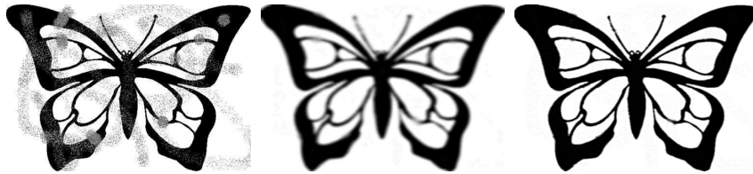
FIGURE 5. Vandalized binary image and the solution of Cahn-Hilliard inpainting with \lambda_0 = 10^9 and switching \epsilon value: u(800) with \epsilon = 0.8 , u(1600) with \epsilon = 0.01
