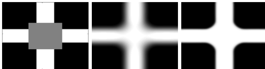
FIGURE 3. Binary image with unknown center and the solution of Cahn-Hilliard inpainting with \lambda_0 = 10^5 and switching \epsilon value: u(600) with \epsilon = 0.1 , u(1000) with \epsilon = 0.01
